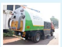
Unit for cleaning the Roads and Wharfs. The equipment has a capacity of 4.0 Cu. M volume and is able to sweep an overall width of 2900 mm in one sweep / pass. The machine has a wandering
